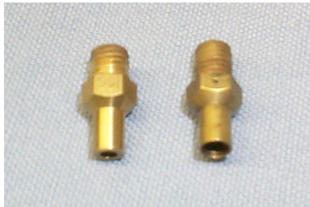
Concentric 2-stroke and 4-stroke needle jets
