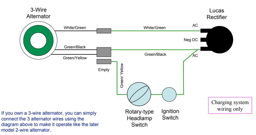
The total power output from a Lucas 3-wire stator is exactly the same as the later model 2-wire stator (120 Watts).
