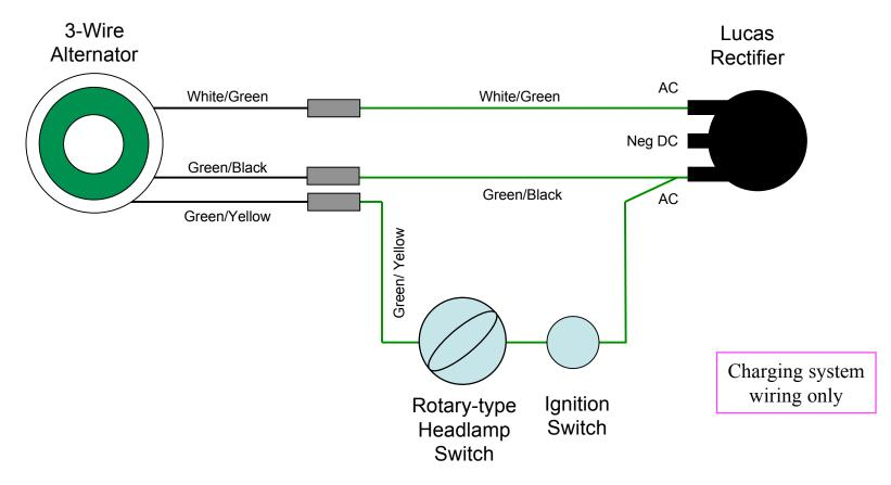
Before the introduction of AC regulators, all 6V and some 12V British motorcycles used the 3-wire Lucas alternator. On those machines the rotary light switch not only turned ON the headlamp, but also activated additional charging coils in the alternator to match the additional load. 1) Now that lights must be ON all the time, and 2) because these older type light switches tend to be more troublesome, it may be better to wire the alternators fully ON, like a post-1968 model.
