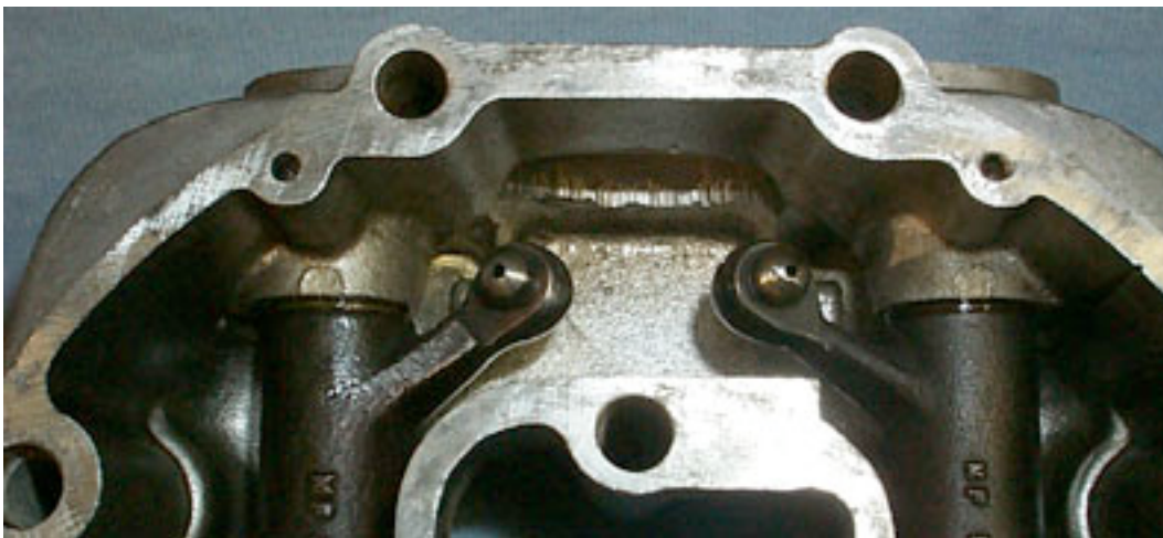
Photo 5. The finished rockers reinstalled in the box
