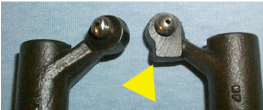
Photo 1. Stock rocker arms and the compression release lug
