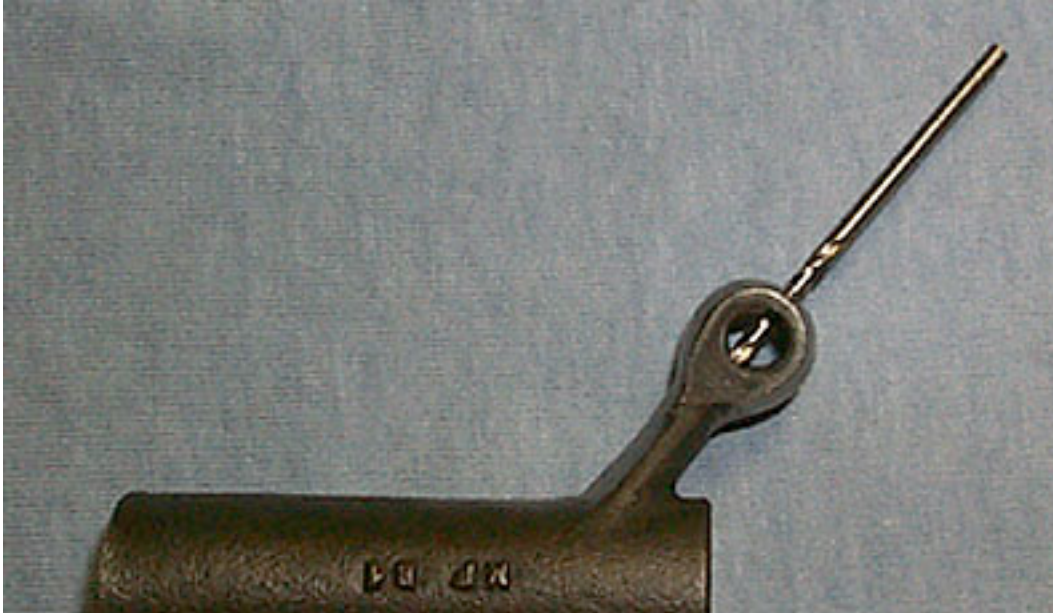
Photo 4. A drill bit shows the oil passage location
